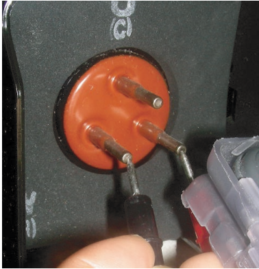
* Measuring resistance between each terminal of compressor
